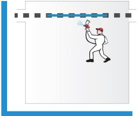
Blue line indicates typical spray area which is limited as it passes in front of the manual sprayer or robot.
