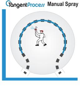
The TangentProcess spray area is 3 times larger with unique non-linear path design as indicated with blue line.
