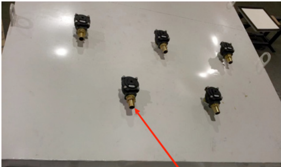
Compressed air feeds from the manifold to each pulse valve.
